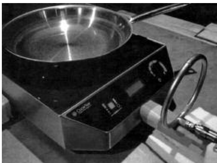
Figure 1. RE101 test for an induction cooking device with loop sensor shown measuring front emissions.
